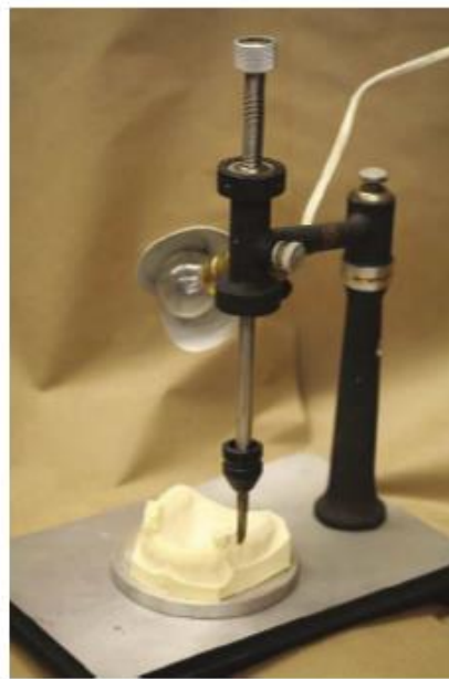
The Jelenko surveyor: Note the spring-mounted paralleling tool and swivel at the top of the vertical arm. The horizontal arm may be fixed in any position by tightening the nut at the top of the vertical arm.
